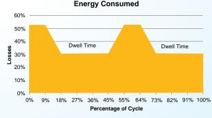
Losses for a 33% duty cycle actuator
