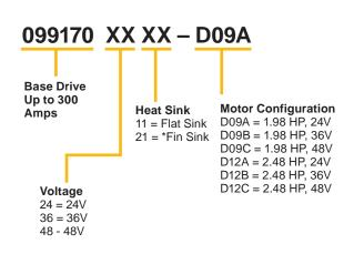
\*Fin style heat sink required forced air for proper inverter cooling.
