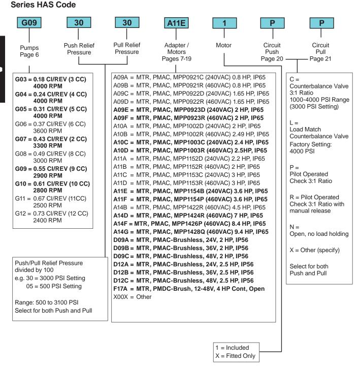
Model code selection for the HAS Power Pack for cylinder type and model selection, see pages 34 for HS2 and 40 for HSR.
