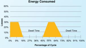
Losses for a 33% duty cycle actuator
