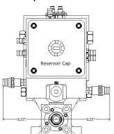
Diagnostic Couplers Package PD361 nipples on Pump Outlets
