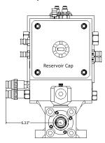
Diagnostic Couplers Package PD361 nipples on Pump Outlets
