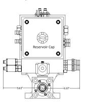
Sensor Package Industrial PD361 nipples on Pump Outlets
