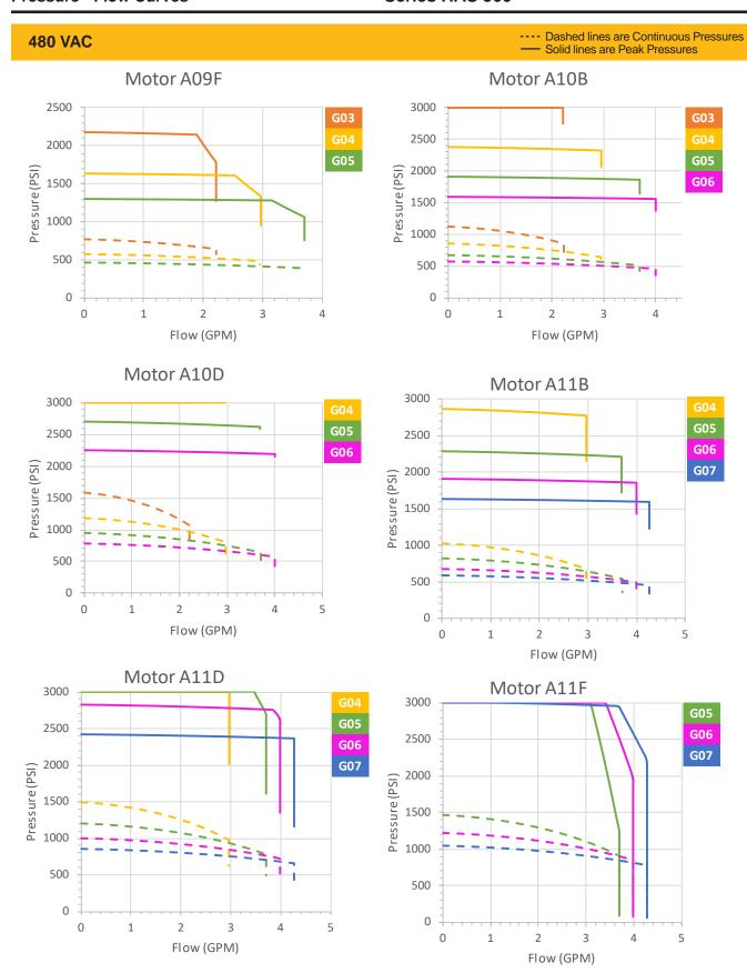
These specifications are based on theoretical motor performance with ambient temperature of 95°F and are not specific to any amplifier. For applications with move time greater than 6 seconds, temperatures above 95°F or motors not listed, please consult factory for sizing.
