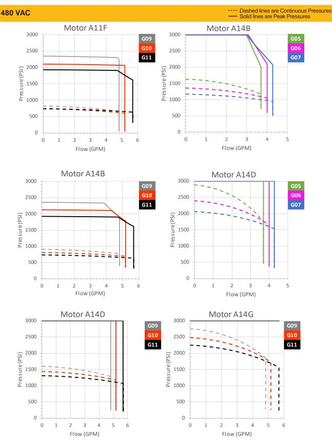
These specifications are based on theoretical motor performance with ambient temperature of 95°F and are not specific to any amplifier. For applications with move time greater than 6 seconds, temperatures above 95°F or motors not listed, please consult factory for sizing.
